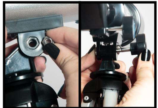
*Figure 6 - Securing Telescope to Tripod with Large Hand Screw and nut.*
