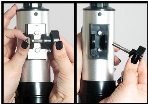
*Figure 5 - Removing the Large Hand Screw and nut from Telescope.*
