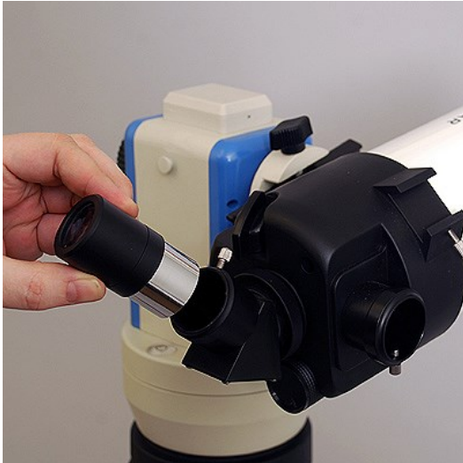
Figure 8 – An eyepiece goes into the angle prism. Be sure to tighten the silver set screw.
