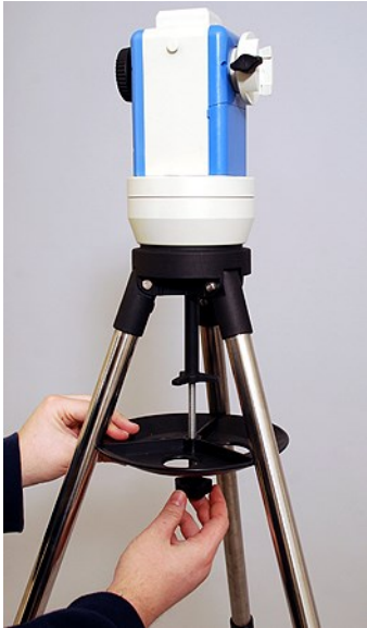
Figure 2 – Attaching the Accessory Tray.
