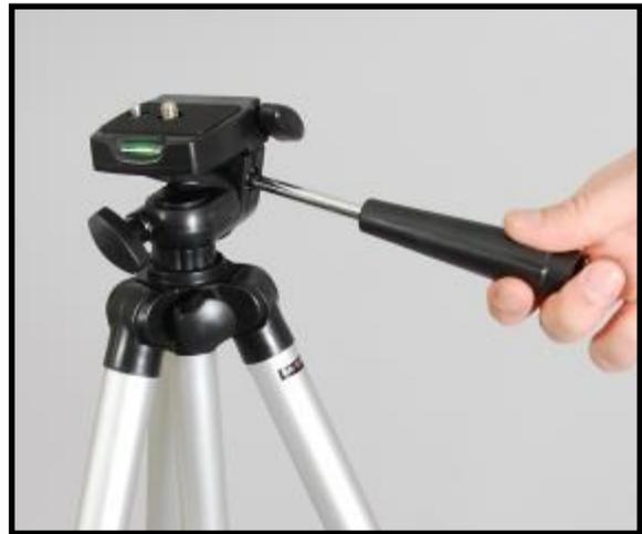
**Figure 2 – Leveling the tripod.**
