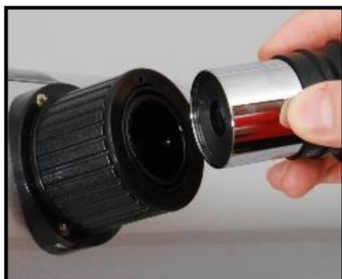
**Step 5** To change eyepieces, simply unscrew the current one to remove it. Then screw in the other eyepiece until snug.
