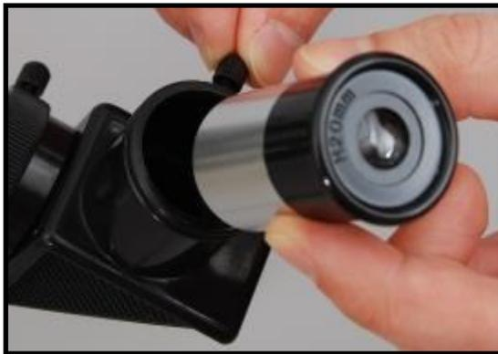
**Step 5** Slide either eyepiece into the angle prism and tighten the thumb screw to secure the eyepiece.
