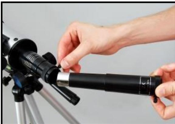
**Optional Step 1** A Barlow lens is an additional part that allows you to multiply your magnification. To use a Barlow lens, first remove the angle prism from the telescope. The Barlow lens inserts into the telescope and tightens with the thumbscrew.
