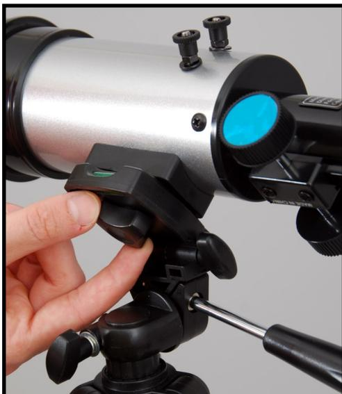
**Step 3** Use the hand screw beneath the tripod's mounting point to screw the telescope in to place. The viewing end of the tripod should be facing away from the handle.
