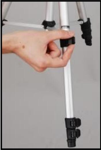
**Figure 1 – Extending the tripod legs.**
