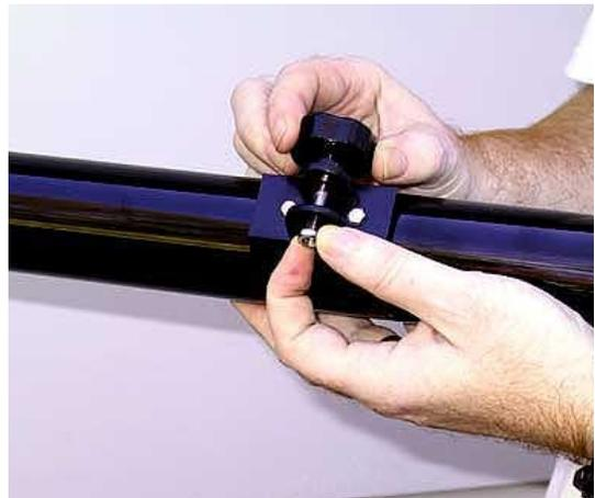
**Figure 3 – Removing the telescope tube securing screw.**
