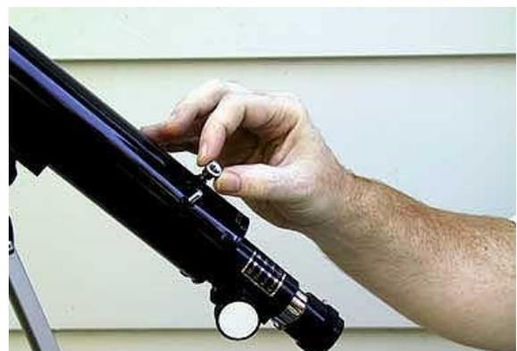
**Figure 7 – Removing the finder scope nuts.**
