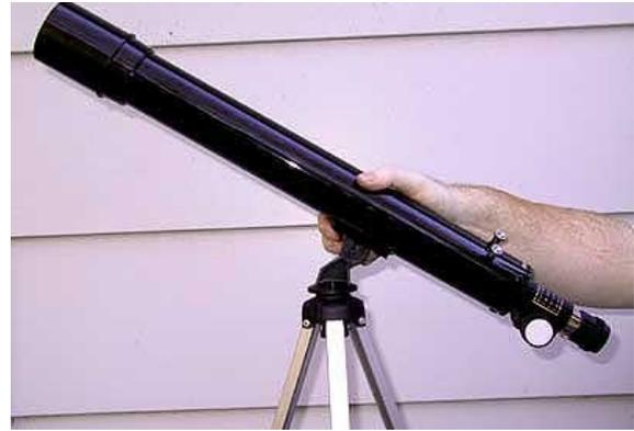
**Figure 5 – Attaching the main telescope tube to the tripod.**
