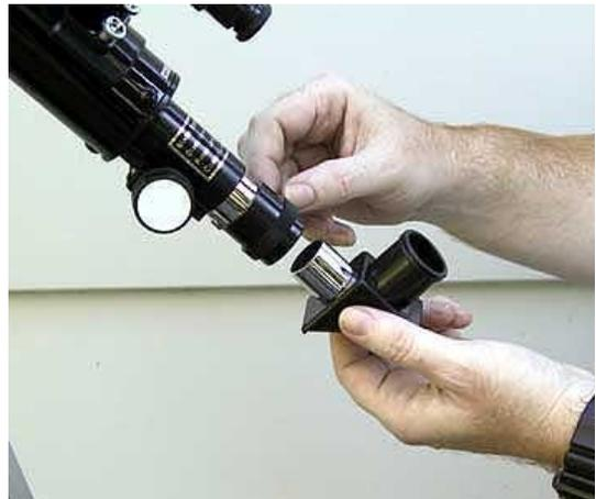
**Figure 9 – Inserting the angle prism.**
