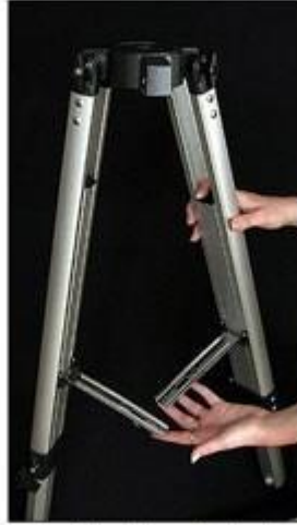
Figure 13 -- Two of the tripod legs attached to the base mount.
