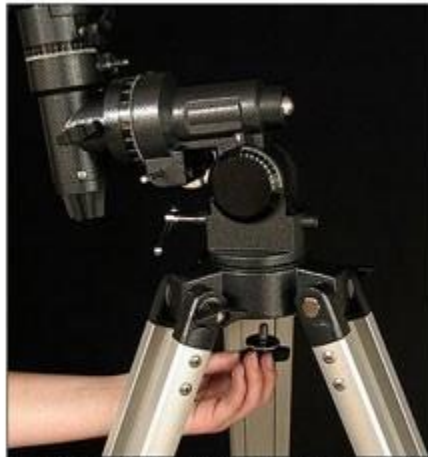
Figure 22 -- Attaching the equatorial mount and tightening it in place.
