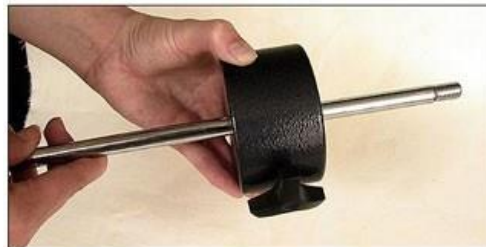
Figure 27 -- Placing the counterweight on the balance shaft.
