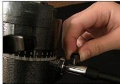
Figure 25 -- Tightening the flexible cable control.
