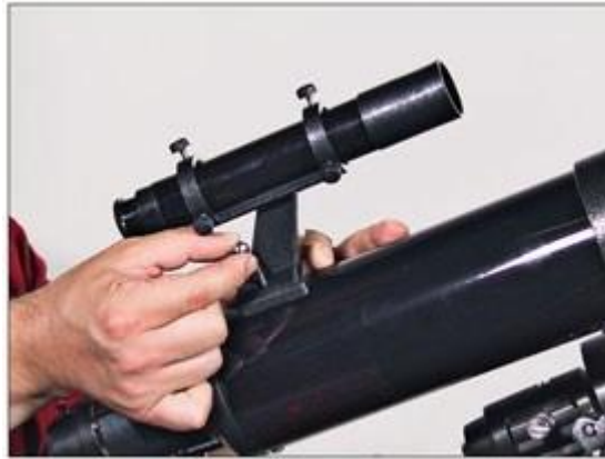
Figure 31 -- Attach the finder scope.
