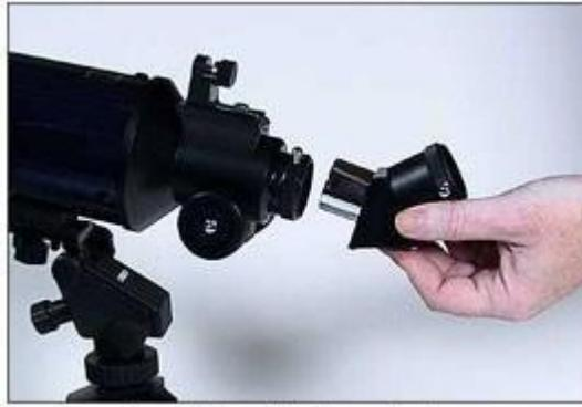
Figure 5 - Inserting the angle prism.
