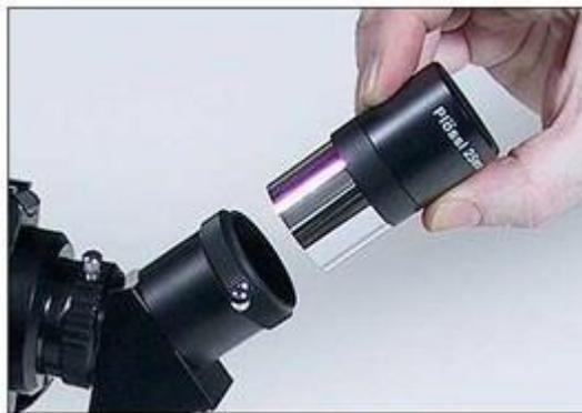
Figure 6 - Inserting an eyepiece.
