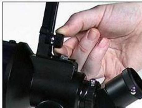
Figure 4 -- Tightening the sighting scope screw.
