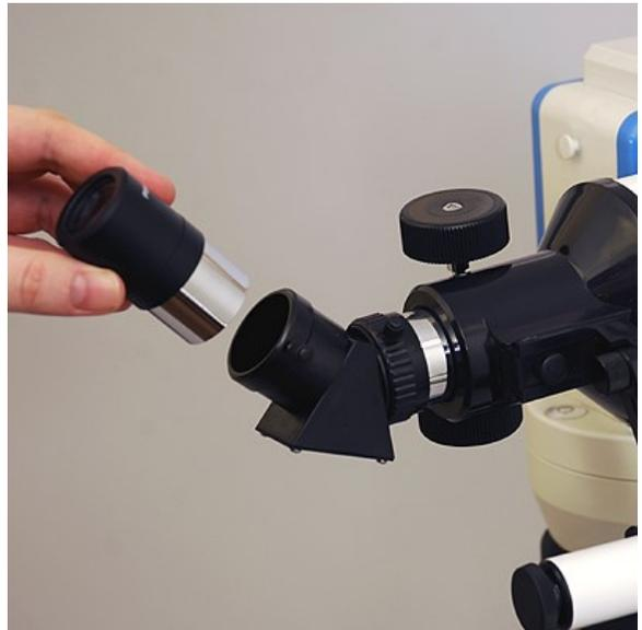
**Figure 9 - An eyepiece goes into the angle prism. Be sure to tighten the set screw.**
