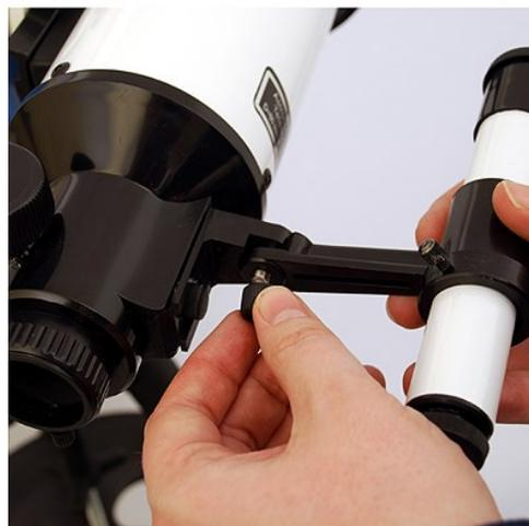
**Figure 7 – The optional sighting scope can be attached to the telescope tube.**
