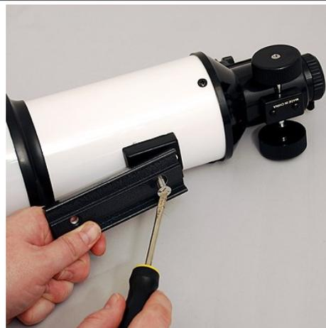
**Figure 5 – Attach the dovetail mount plate to the telescope.**
