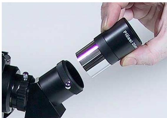
**Figure 6 – An eyepiece goes in the angle prism.**
