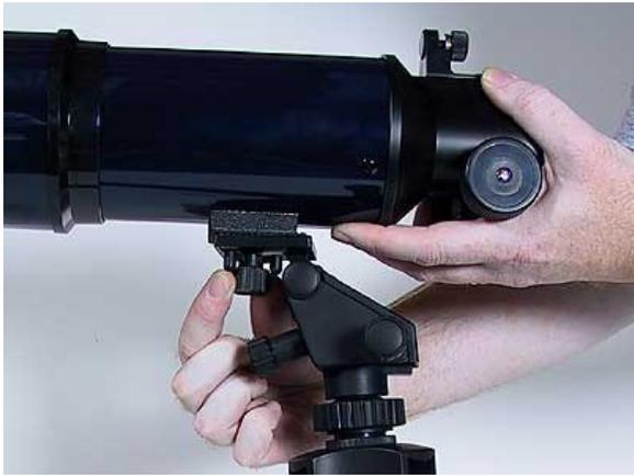
**Step 2** >Attach the main telescope tube to the tripod head using the photo bolt screw as shown in Figure 2.
