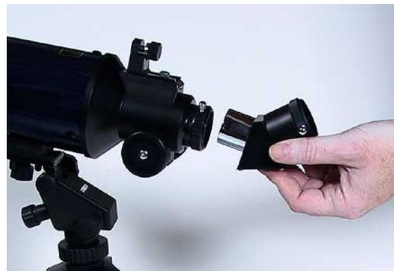
**Figure 5 - Inserting the angle prism.**
