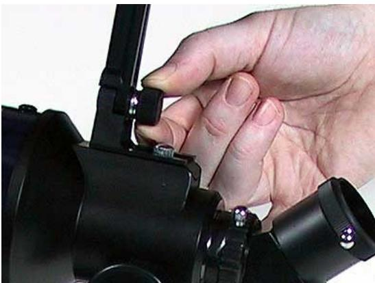
**Step 4** Tighten the sighting scope in place with the screw provided.
