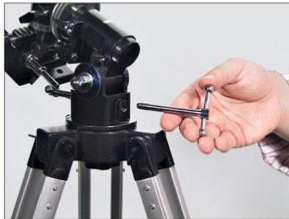
Figure 15 -- Attaching the polar axis screw.
