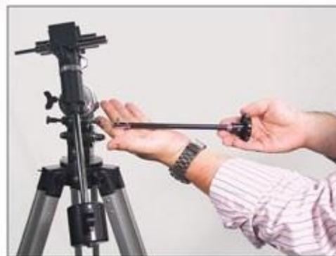
Figure 19 – Attaching the RA flexible cable control.
