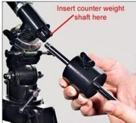
Figure 17 – Attaching the balance shaft and counterweight to the equatorial mount.
