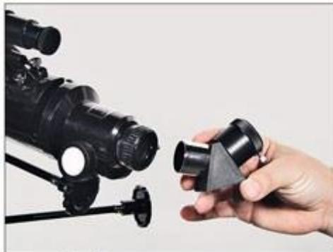
Figure 22 -- Attach the angle prism to the main telescope tube.
