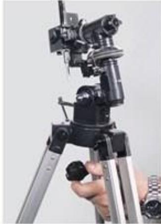
Figure 14 -- Attaching the equatorial mount and tightening it in place.
