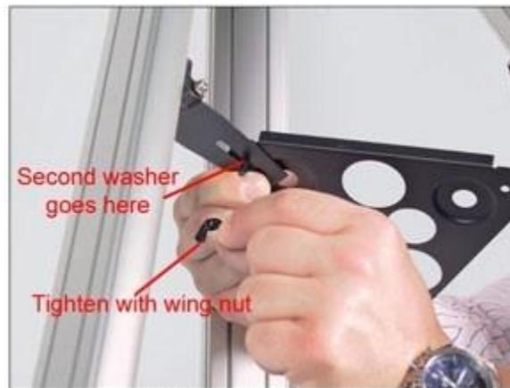
Figure 11 -- Installing the Accessory Tray.
