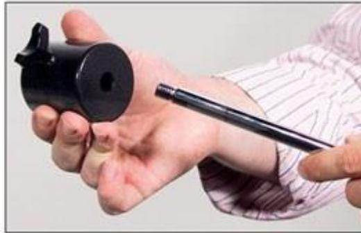
**Figure 16** -- Placing the counterweight on the balance shaft.
