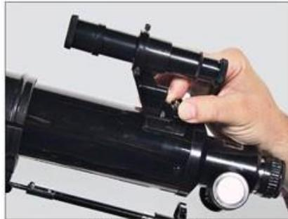
Figure 21 -- Attaching the finderscope.
