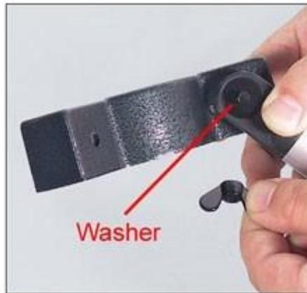
Figure 8 -- The wing nut goes on the end to tighten the assembly.
