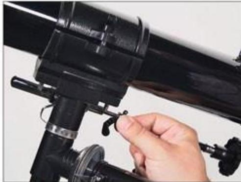
Figure 20 -- Attaching the telescope to the mount.
