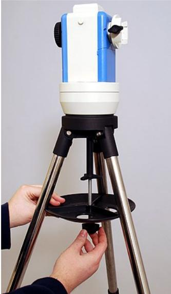
**Step 2** Attach the Accessory tray to the tripod as shown in Figure 2.
