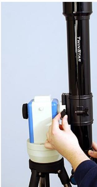
**Step 4** Your 70mm telescope attaches directly to the iOptron Mount and locks in place with a set screw: **IMPORTANT:** Be sure that the mounting “body belts” are positioned low enough on the telescope tube so that the focusing knobs can rotate clear the tripod legs when the telescope is the vertical “parked” position. This means the body belt around the center of the telescope should be roughly 2/3 of the way down the telescope as shown in Figure 4.
