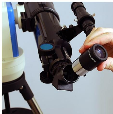
**Figure 7 –** An eyepiece goes into the angular prism. Be sure to tighten the set screw.
