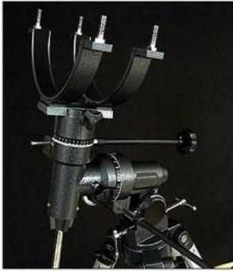
Figure 31 -- Attaching the body belt to the equatorial mount.
