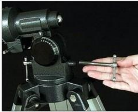
Figure 23 -- Attaching the polar axis screw.
