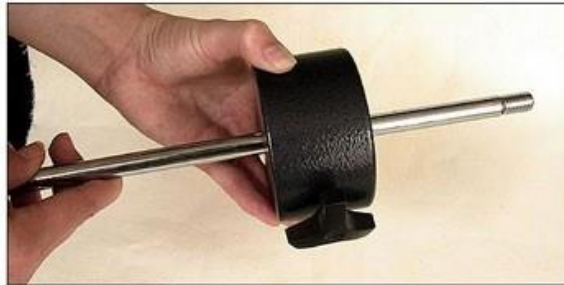
Figure 27 -- Placing the counterweight on the balance shaft.
