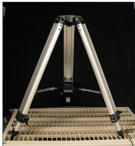
Figure 20 -- The finished tripod assembly with attached accessory tray.
