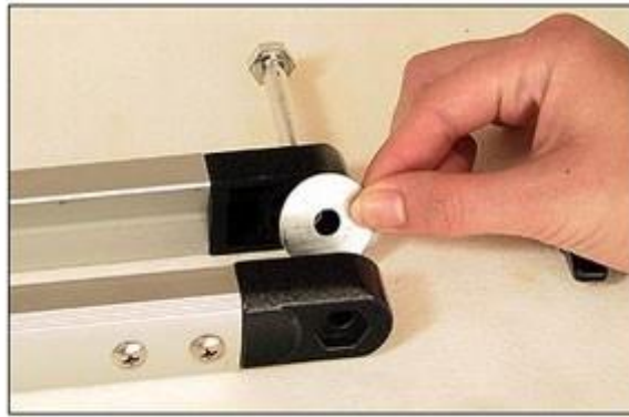
Figure 7 -- Placing the first large flat washer on the tripod assembly.
