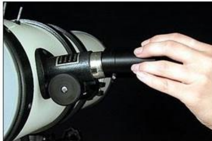
Figure 33 -- Attaching the eyepiece adapter.
