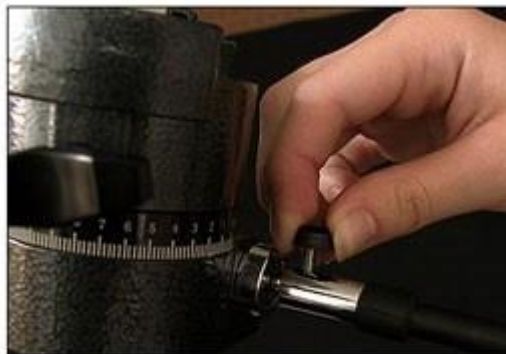
Figure 25 -- Tightening the flexible cable control.
