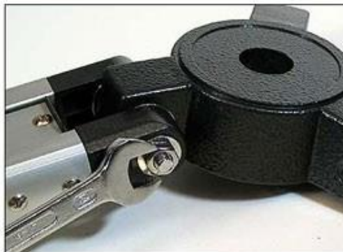
Figure 12 -- Tightening screw on completed tripod assembly with base mount.
