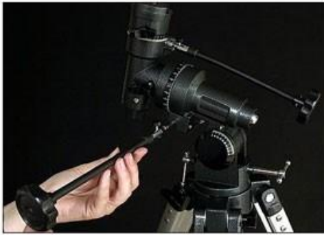
Figure 26 -- Attaching the right ascension flexible cable control.
