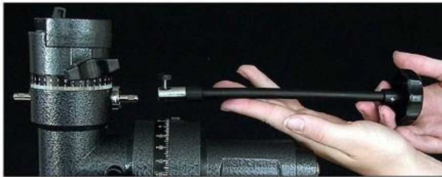
Figure 24 -- Attaching the declination flexible cable control.
