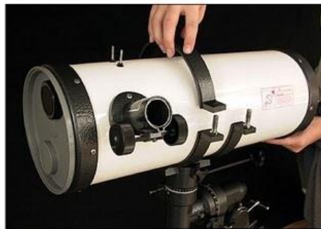
Figure 32 -- Attaching the body belt to the main tube.
