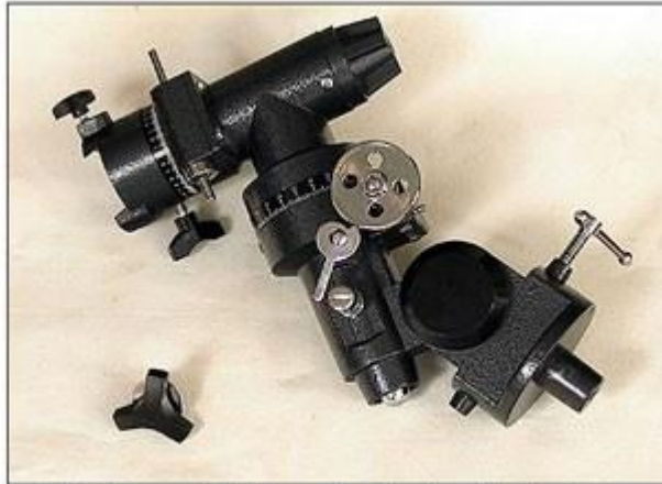
Figure 21 -- The equatorial mount and horizontal axis clamp screw.
