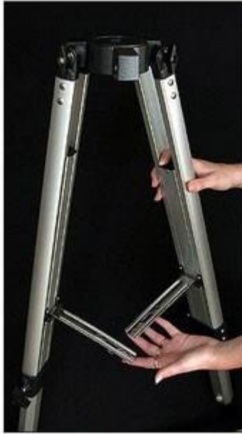
Figure 13 -- Two of the tripod legs attached to the base mount.
