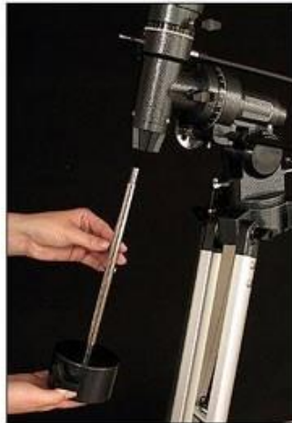
Figure 28 -- Attaching the balance shaft and counterweight to the equatorial mount.
