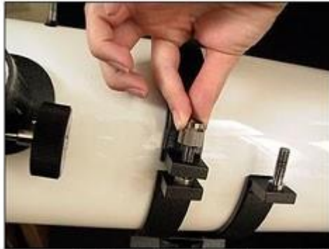
Figure 29 -- Unscrewing the body belt from the main telescope tube.
