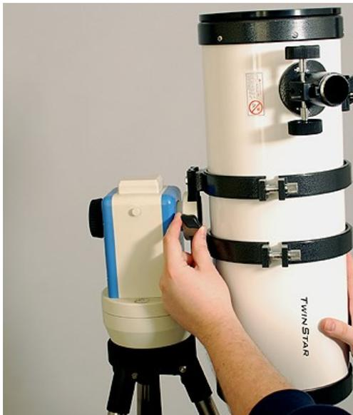
**Step 4** Your 6 inch telescope attaches directly to the iOptron Mount: **IMPORTANT:** Be sure that the mounting “body belts” are centered on your telescope tube. If your telescope is not balanced in the center of the tube, you will damage the motor inside the mount.
