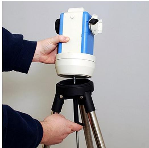
Figure 1 – Attaching the SmartStar Cube.
