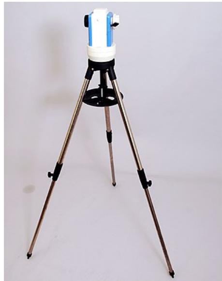
**Figure 3 – The completed iOptron Smart-Star tripod and mount.**
