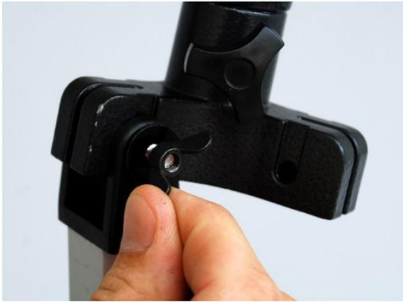
**Step 2** Attach all three legs to the center connector that will hold the telescope as shown in Figure 2.
