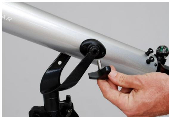
**Figure 5 – Attach the telescope to the mount using the two tri-wing screws.**
