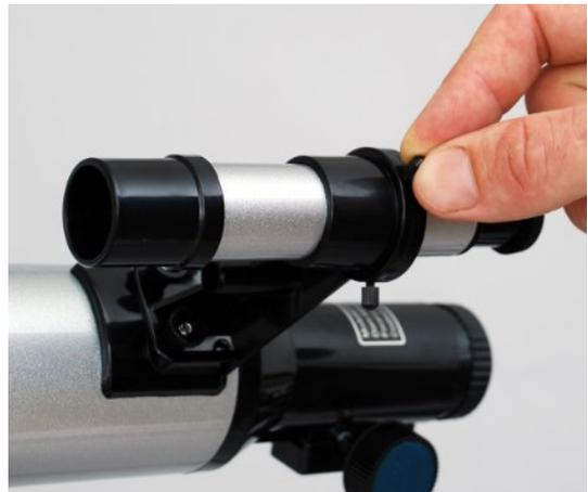
**Figure 9 – Securing the sighting scope with the hand screws.**
