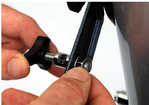
**Figure 6 – Screwing in the pitching clamp handle screw.**
