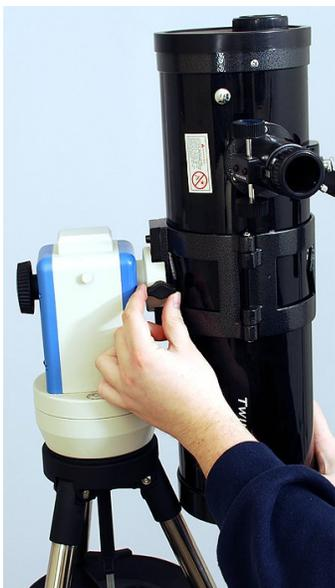
**Step 4** Your 4.5 inch telescope attaches directly to the iOptron Mount: **IMPORTANT:** Be sure that the mounting “body belts” are centered on your telescope tube. If your telescope is not balanced in the center of the tube, you will damage the motor inside the mount.
