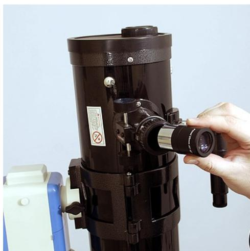
**Step 6** Finally, insert one of your eyepieces into the focusing tube, as shown in Figure 6, and you are ready to begin observing. Be sure to tighten the set screw that holds the eyepiece in place.
