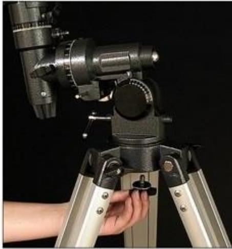
Figure 5 - Attaching the equatorial mount and tightening it in place.
