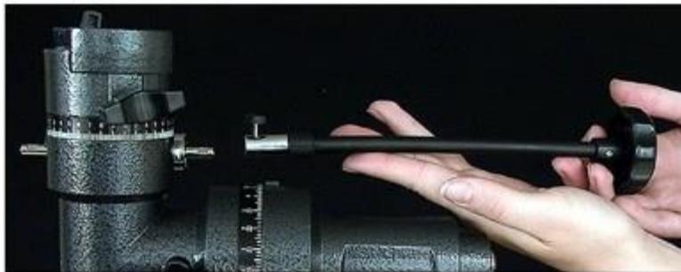
Figure 7 - Attaching the declination flexible cable control.
