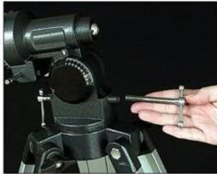
Figure 6 - Attaching the polar axis screw.
