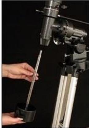
Figure 11 -- Attaching the balance shaft and counterweight to the equatorial mount.
