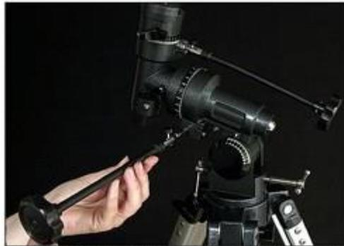
Figure 9 - Attaching the right ascension flexible cable control.
