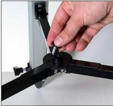
Figure 2 - Removing the Accessory Tray Screw.
