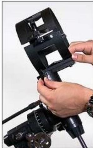
Figure 12 -- Attaching the body belt to the equatorial mount.
