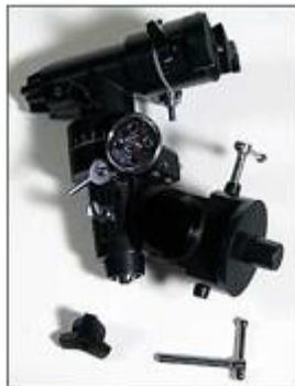
Figure 4 The EQ mount, horizontal axis clamp screw, and polar axis screw.
